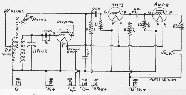
Fig. 2. Detector and Two Steps Resistance Amplifier Without Leaks
