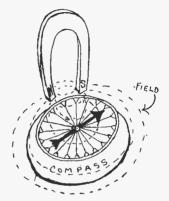
Fig. 3. Magnetic Field from Poles
