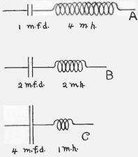
Fig. 2. Coil and Condenser for Tuning
